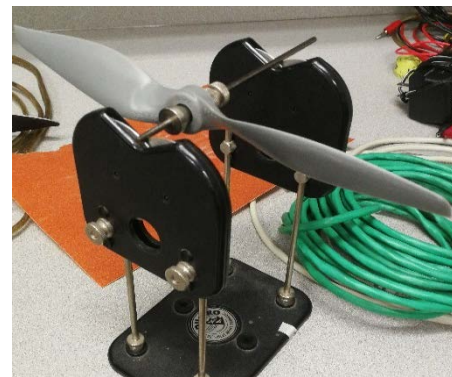
Figure 28. Propeller balance stand.
