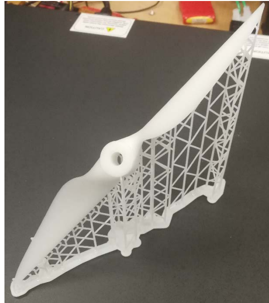
Figure 22. Propeller just printed with the stereolithographic machine.
