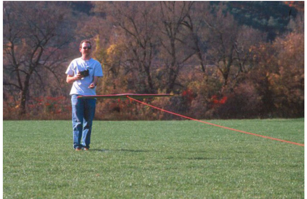
Kyle test flying the Bat using a bungee launch. Because of the high speed of the launch, over-controlling was easy. Easing up on the stick made a big difference. OK, off to the slope! Photo by Dave Garwood.
